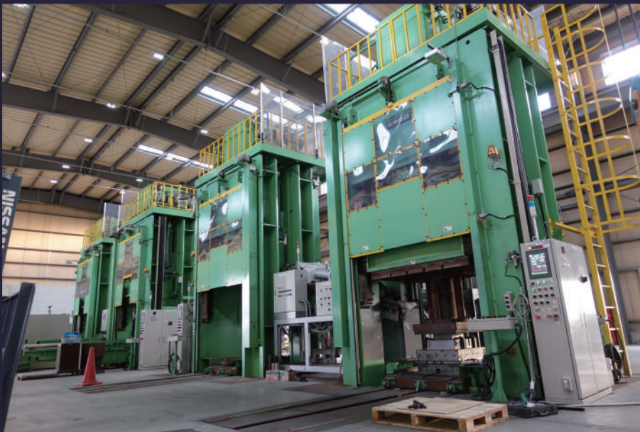
High Pressure Press Machines (9 machines owned) for Squeeze Casting
