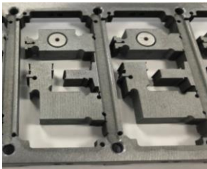
Reflow positioning jig
